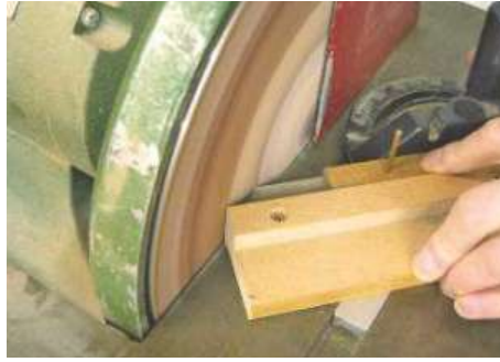
▲ Pic 6 Dominic roughly cut the point at the end of the blade using a disc sander and mitre gauge
